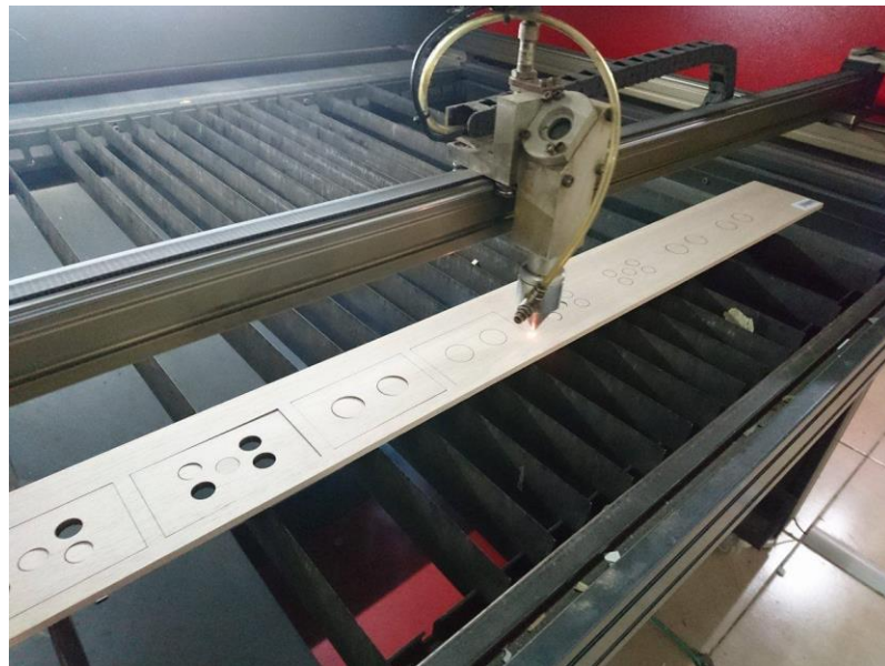
Figure: 40 Laser Cut of the Wooden Plate
